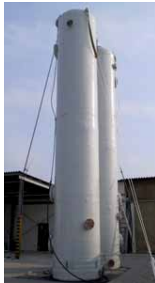
STRIPPING TOWERS height 11 m
